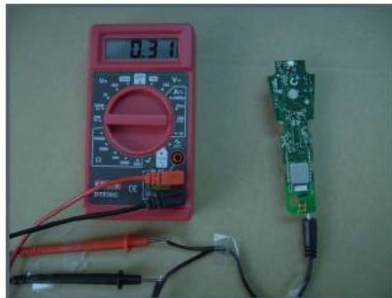
Fig 5. Charging current checking
